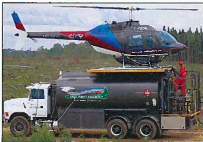
Loading a spray aircraft with modern leak-proof systems and appropriate personal protective equipment.
