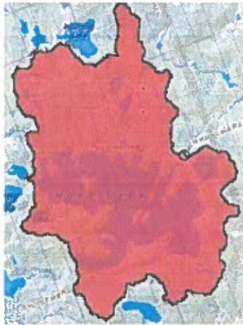
Figure 1: Watershed drainage area that outlets through the Horn Lake culvert at Highland Road. The approximate drainage area is 20km 2 .
