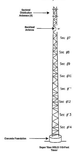
Note: The configuration and mounting of antennas on the tower mast may not be exactly as shown.
