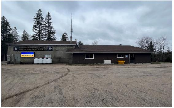
Brick left section is approximately 11 metres in length and 4.5 metres in height. Siding right section is approximately 18 metres in length and 2.47 metres in height.
