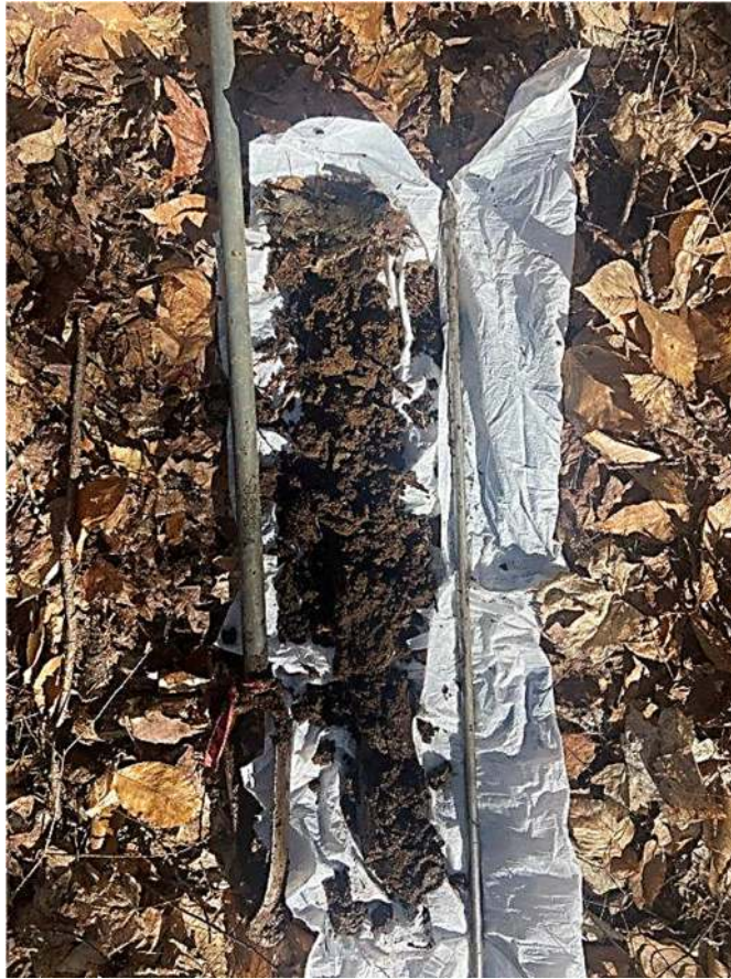
Photograph 11. Soil profile from one of several areas within proposed building envelope that would be suitable for a sewage disposal bed (April 10, 2024).
